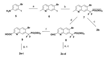
Scheme 1. Reagents and conditions: (a) chloranil, concd HCl in *i*-PrOH at reflux, then crotonaldehyde in *i*-PrOH via syringe pump; (b)  $(EtO)_2P(O)CF_2ZnBr$ , CuBr, DMF, 60 °C; (c) TMSBr, DCM, rt and then co-evaporate with water/ethanol (3×); (d) SeO<sub>2</sub>, ethanol, reflux; (e) ArCH<sub>2</sub>P<sup>+</sup>Ph<sub>3</sub>Br<sup>-</sup>, LiHMDS, THF, -78 °C—rt; (f) AgO, MeOH, rt; (g) EDCI, RNH<sub>2</sub>, TEA, trace DMAP, DCM, rt.
