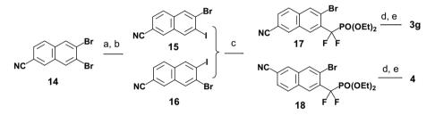
Scheme 3. Reagents and conditions: (a) *n*-BuLi, TMSCl, THF,  $-78 \degree$ C; (b) ICl, DCM, rt; (c) (EtO)<sub>2</sub>P(O)CF<sub>2</sub>ZnBr, CuBr, DMF, 45 \degreeC; (d) TMSBr, DCM, rt and then co-evaporate with water/ethanol (3×); (e) NH<sub>4</sub>OH, MeOH, rt.
